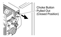
Figure 21 - Choke Button Closed (Model RGH11000AIE Only)
